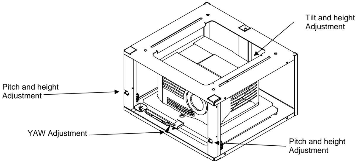
1. Begin by determining the exact mounting position of the AVStack frame. Span structural beams with a structural channel if points are not located precisely above (4) mounting points.
