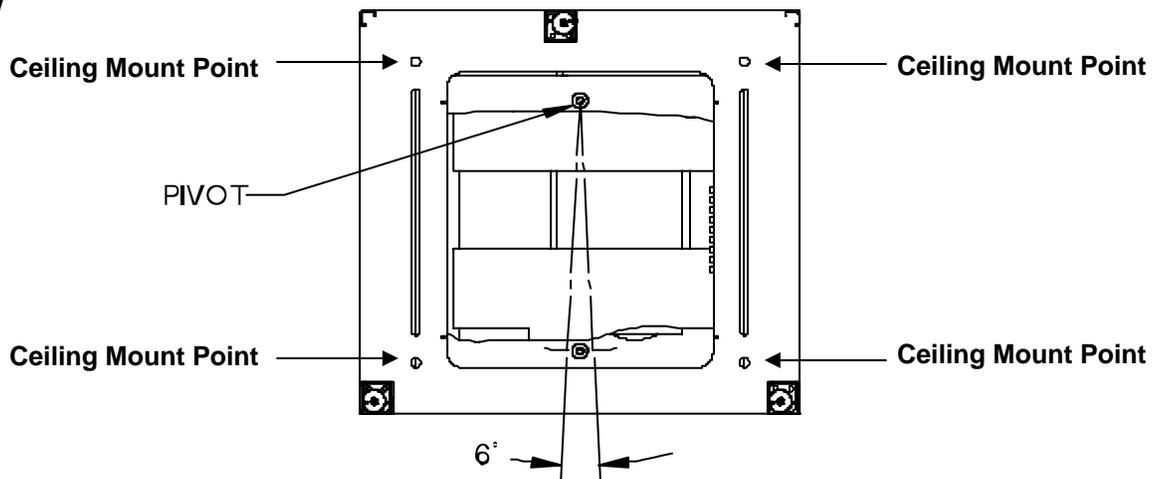
2. Use 3/8" threaded rod to attach to the (4) mounting points on the AVStack. These points are located towards the corners of the frame. Be sure to use split lock washers, flat washers and upper and lower nuts. If mounting to truss, use properly-rated c-clamps or cheeseboroughs. The mounting hardware can attach to the slots to canter on an angle.
